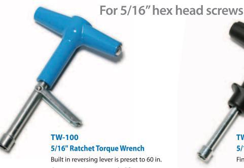
Built in reversing lever is preset to 60 in. Ibs. torque. Recommended for Fernco Couplings and other banded Fernco products. It has a chrome plated shank, with all metal construction.
