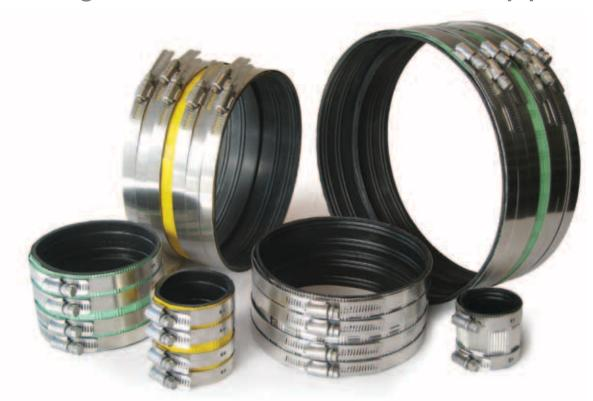
Choose the No-Hub Coupling with the patented shield design that provides maximum transfer of pressure from the clamps - to the gasket - to the pipe. Engineered to connect no-hub cast iron pipe in applications replacing the less-efficient hub and spigot.
