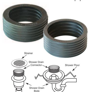
Shower Drain Connectors connect 2" DWV plastic, Sch. 40, steel or X.H. (extra-heavy) cast iron pipe to shower drain bodies. They reduce the time and cost of installation because no special tools, gluing, threading or lead caulking are required.
