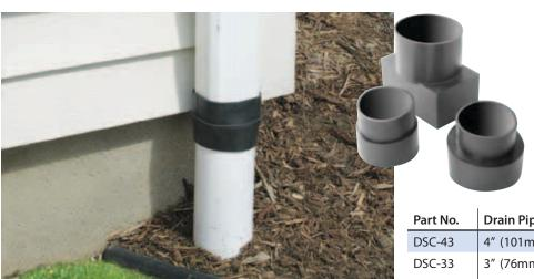
Fernco Flexible Downspout Connectors stretch easily over most common downspouts and drain pipes to seal out problem-causing debris and pests. Installation is fast and simple. For use with aluminum, steel or plastic downspouts and cast iron, spiral, corrugated or plastic drain pipe.
