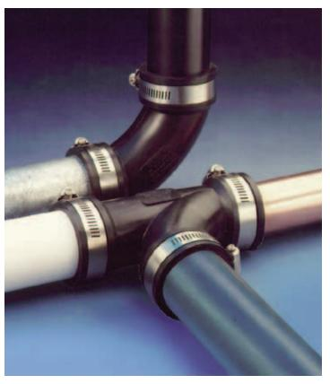
Qwik Tees and Ells let you make 90° connections of all common household drain, waste and vent pipes quickly and easily without using special tools or fittings. Because they're exceptionally flexible and extra long, they're the ideal replacement for fittings cut out at the joint during alteration or repair. Reducing sizes are made with separately supplied Qwik Bushings.
