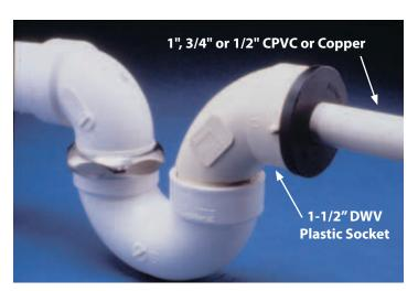
These one piece connectors are designed for quick, easy connections. With a simple press fit (no tools needed) they connect 1", 3/4" or 1/2" CPVC and copper pipe to 1-1/2" DWV Schedule 40 plastic sockets (ABS or PVC).
