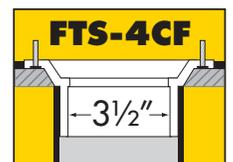
**3x4 Flange / Slab Flange INSIDE 4" Drain Pipe**
