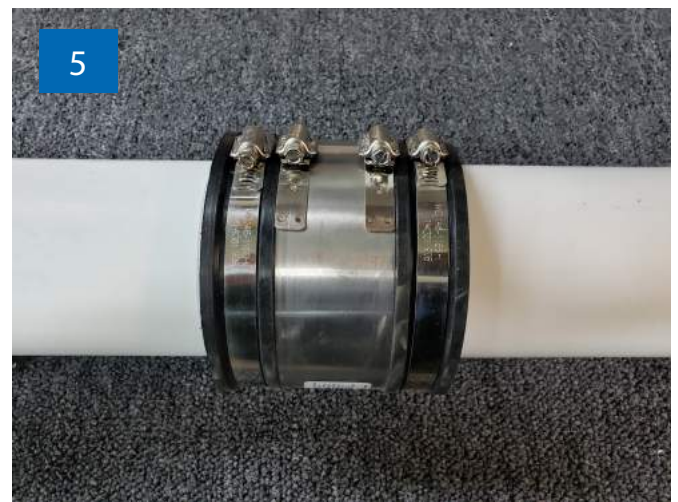
Install the coupling. Tighten band to 60 inch pounds. Test for leaks.
