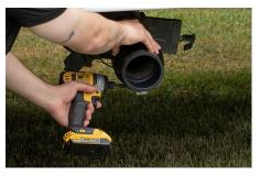
**Step 3** Install the larger end of the 4" x 3" gate valve adapter onto the bushing and tighten the band securely. **DO NOT** overtighten.
