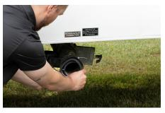
**Step 2** Install the gate valve bushing onto the RV drain by aligning each opening with the tabs of the bayonet fitting.
