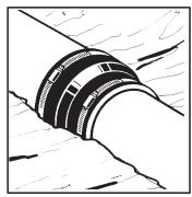
Pressure test\* before backfilling or concealing joint. Bed and backfill properly.
