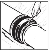
Tighten clamps to 60 inch-lbs. of torque.
