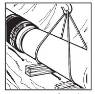
Insert new pipe or fitting then slide flexible coupling over new and old pipe ends.
