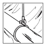
Fernco flexible couplings can be used to couple pipe at a break or lateral insertion.
