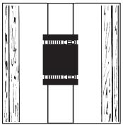
Support pipe and test\* for leaks before concealing joint.
