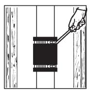
Tighten clamps to 60 inch-lbs. of torque.
